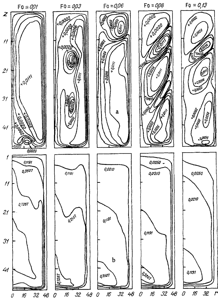
Fig. 3. Distribution of the stream function (a) and isotherms (b) in the liquid of a rotating tank: Gr = 1000 ; Re = 2000 ; \lambda = 4 ; Pr = 1 .
